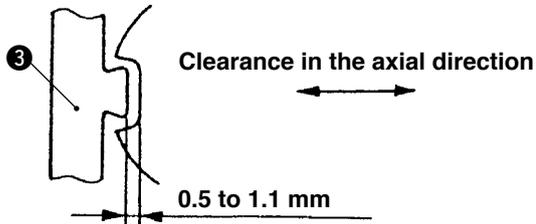
2. Adjust the longitudinal position of the bobbin case opening lever ③ so that the needle enters almost the center of the bobbin case opening lever ③.
