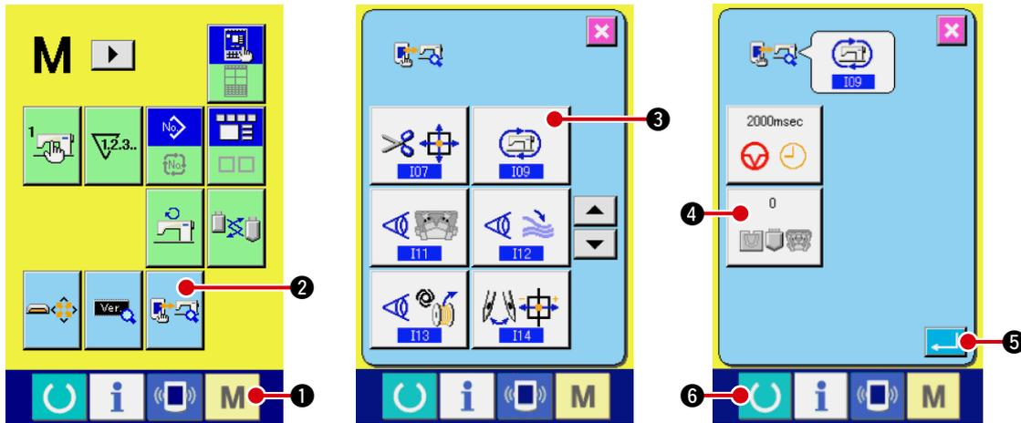
1. Turn the power ON. Then, keep **M** key ① held pressed to display the adjustment screen.
