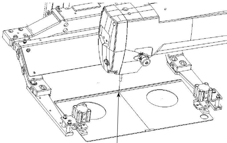
Needle tip aligns with the center marker dot.
