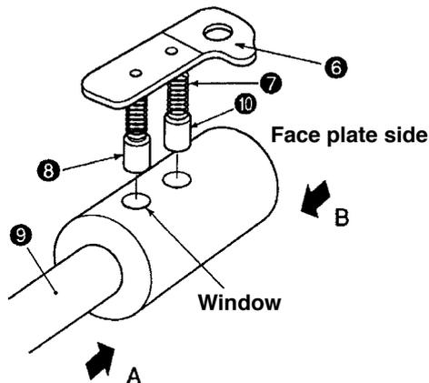
4. Rotate the main shaft ⑨, and confirm that plunger ⑧ moves up or down.
