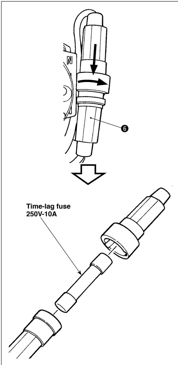
2. If it turns with pushing the fuse case ⑥ in the direction of the arrow, the fuse case ⑥ will open.
