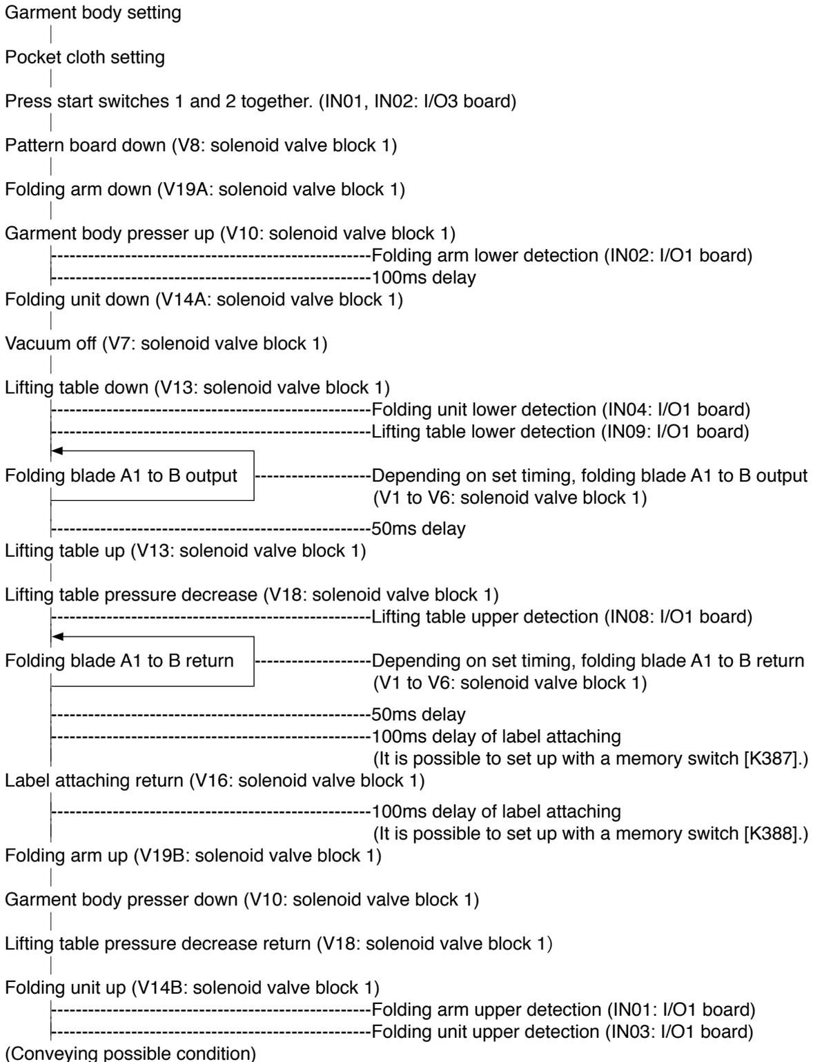
\* Numbers in parentheses are solenoid valve numbers (Vxx) and automatic switch numbers (INxx).
