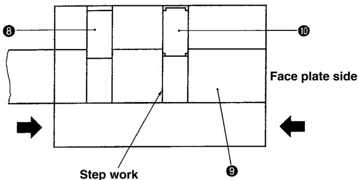
5. If the plunger does not move up or down, strike the bushing from direction A or direction B with a brass bar or the like so that the step work on the main shaft ⑨ cannot be seen from the window.
