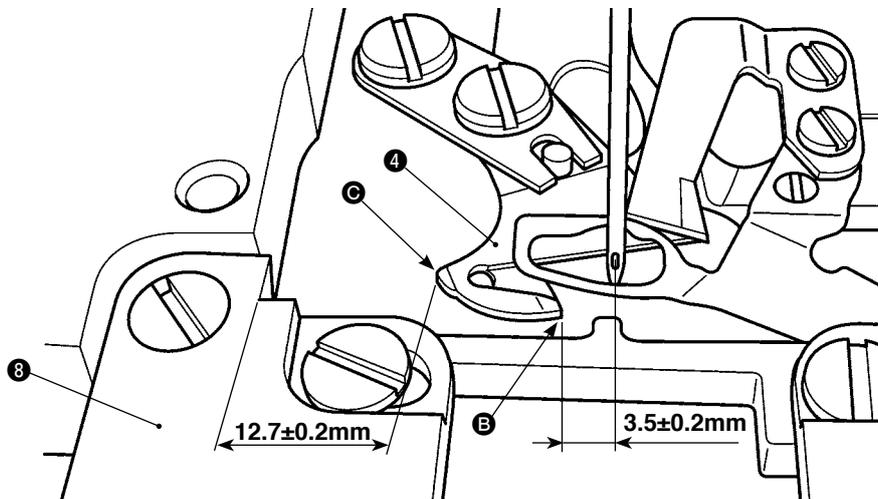
In addition, the position of moving knife **4** can also be adjusted properly by adjusting the distance from the notch of bobbin case opening lever mounting plate **8** to top end **C** of moving knife **4** to  $12.7 \pm 0.2$  mm.
