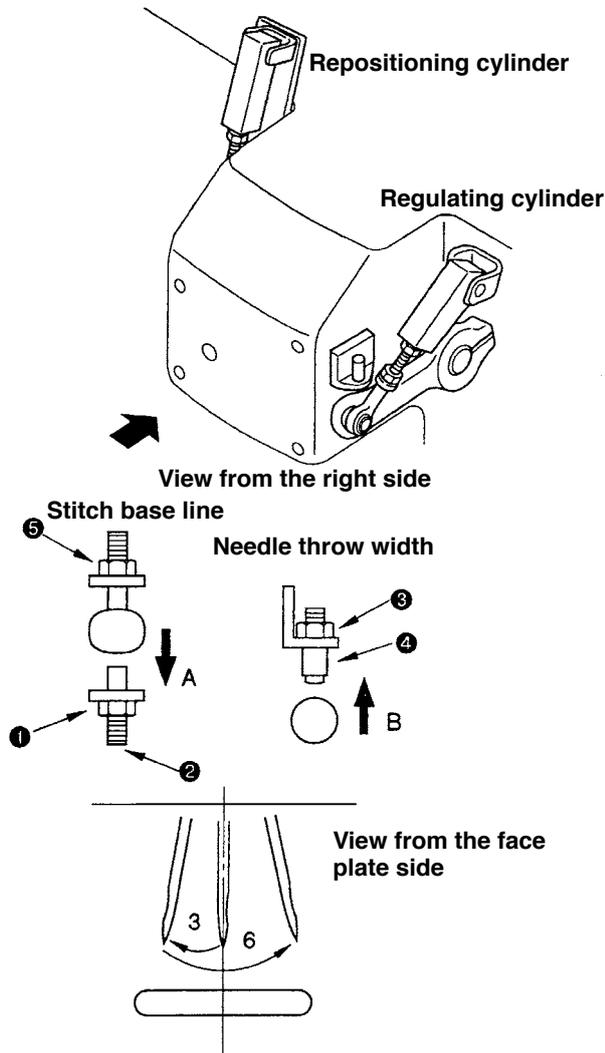
Example) Changing the current 2 mm stitch base line and 4 mm needle throw width to 3 mm stitch base line and 6 mm needle throw width
