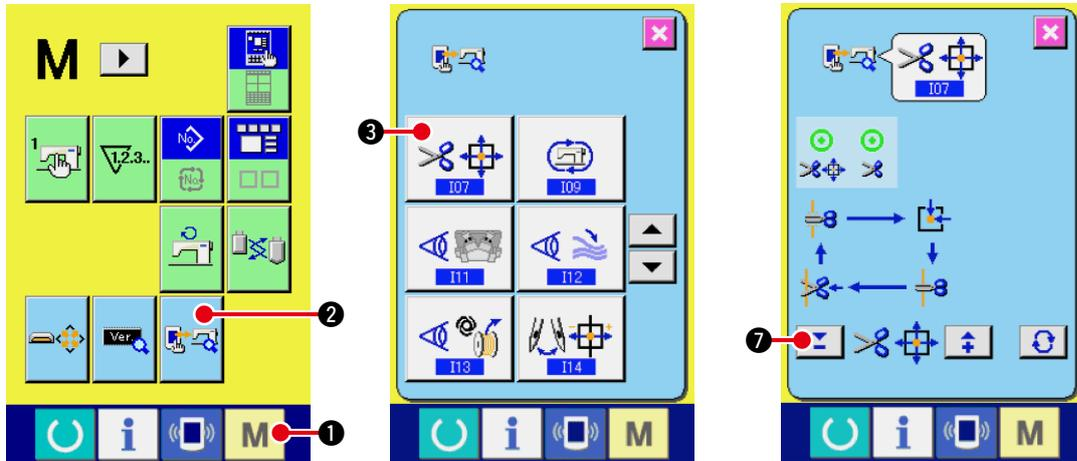
1. Turn the power ON. Then, keep **M** key **1** held pressed to display the adjustment screen.
