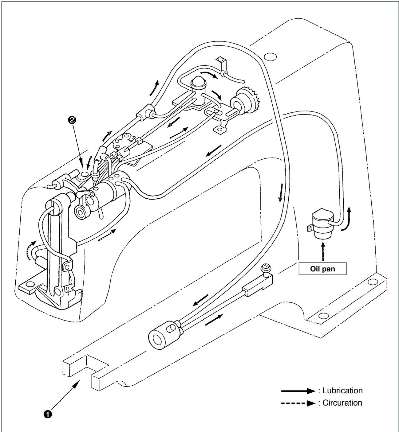
When you first use your machine after set-up or after an extended period of disuse, pour approximately 10 cc oil to hook components ❶ and oil hole (lubrication hole) ❷ of main shaft front bushing.
