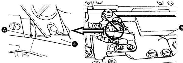
5. At this time, press
