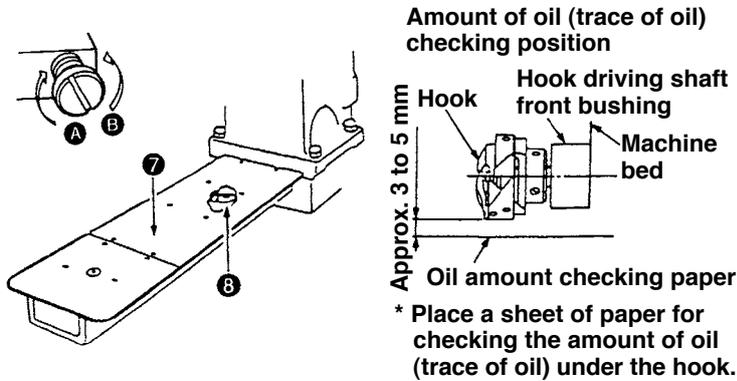
1. Remove throat plate ⑦. Turn oil amount adjustment screw ⑧ that is mounted on the hook lubricating manifold in the "+" direction (direction ④) to increase the amount of oil (trace of oil), or in the "-" direction (direction ⑤) to decrease it
