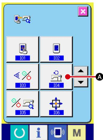
**5) Main motor rpm check (I04)**
