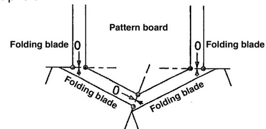
Loosen the folding blade setscrews or the folding cylinder setscrews and adjust so that the relations between the pattern board and the folding blades are as shown above.
