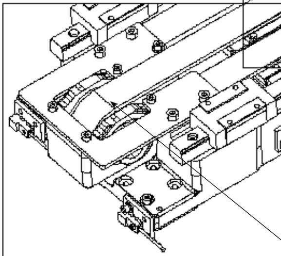
All XY driving pulley and trailing pulley setscrews: ④
