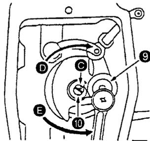
1. Adjust the amount of oil to be fed to the thread take-up lever and needle bar crank unit ⑨ by turning oil amount adjustment screw pin ⑩.
